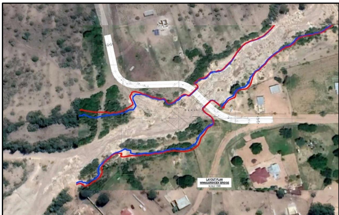
Figure 2. Alignment of the proposed bridge
