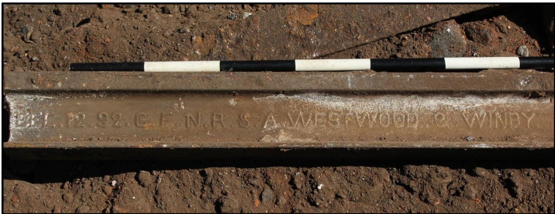
Figure 21. A section of a Westwood & Winby track, showing the date ('92), GFNR, as well the company name (GFNR = probably a misprint for GNFR - Goods Not For Resale? - an important statement made in the production and sale of material in especially an industrial context.)
