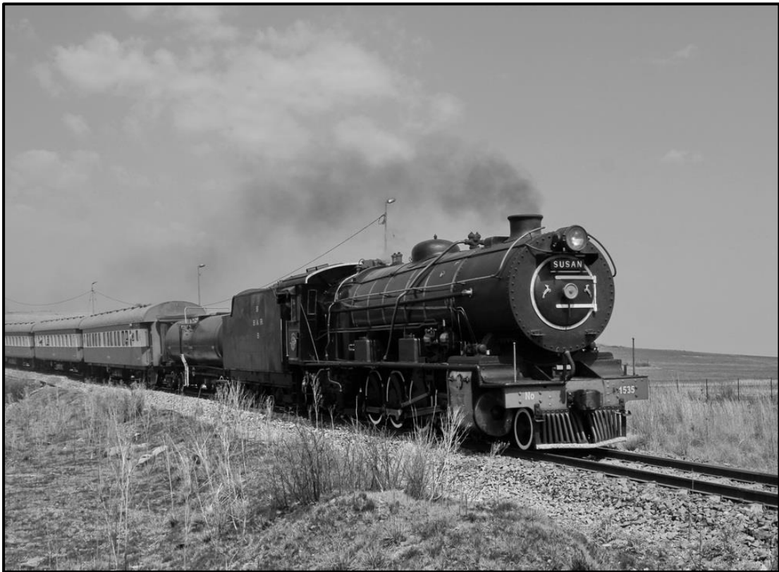
A SAR Class 12AR (a reboilered Class 12A) locomotive with a 4-8-2 configuration, mostly used for heavy hauling during the 1970s and 1980s. The railway track is classified as Cape gauge (3ft 6in)
