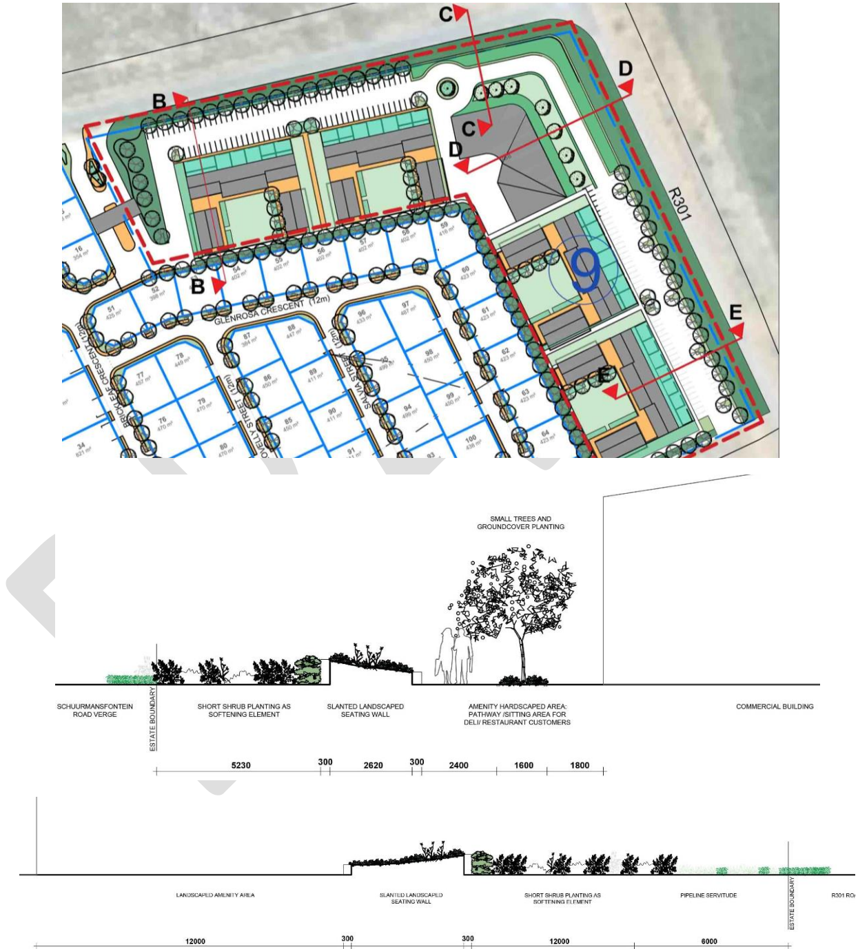
Figure 48: Landscape plan and cross sections through the R310 Scenic route interface with the Mixed-Use component (Viridian Consulting, 2022)
