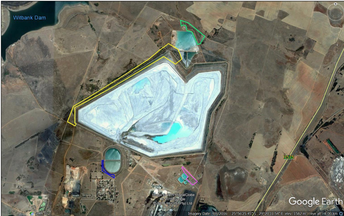
Figure 3: Google Earth image showing the proposed servitude footprint areas for the seepage interception drains (yellow, green, blue and pink polygons) (Map provided by Nemaï Consulting, 2017).
