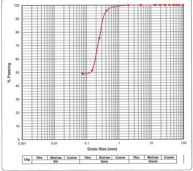
ck Red Line is the Grading Curve (COLTO Classification = Cannot be Determined) (TRH 14 Classification = Poorer than G1
