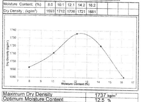
ptimum Moisture Content 12.5 % shows test results are pertinent only to the samples received and tested at the laboratory. This report shall not be reproduced. except in full, without the prior consent of SOILCO MATERIALS INVESTIGATIONS (PTY) LTD
