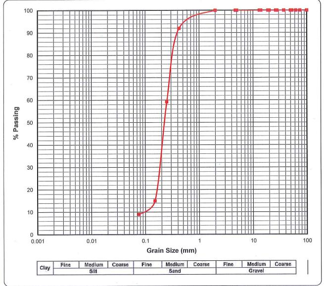
Thick Red Line is the Grading Curve (COLTO Classification = G7 (#)) (TRH 14 Classification = G7)
