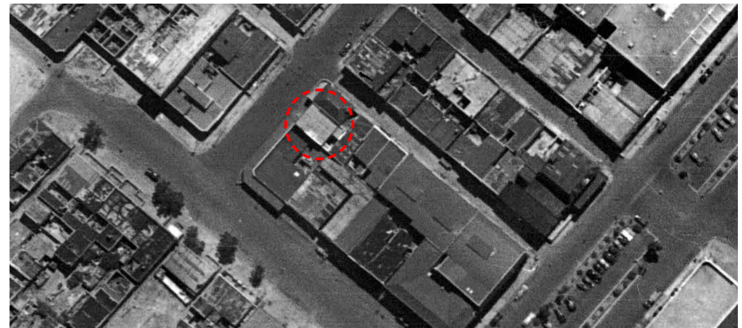
Figure 57. 1945 aerial image light-well enclosed, roofing appears new. Rear outbuildings adjoining east party wall in place. Site circled in red (NGI)
