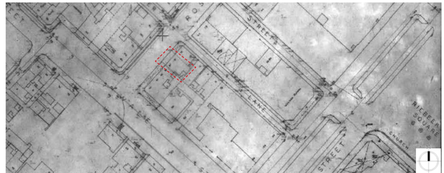
Figure 56. c1944 480 Series survey shows light-well opening, rear north extension and outbuilding (CoCT Historical Imagery)
