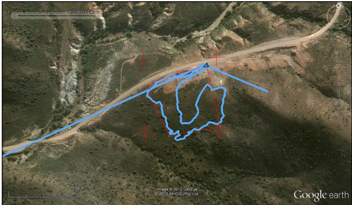
Figure 2: Google earth image showing the proposed extension of the existing borrow pit 30 and tracks of the field survey. Please note that the straight blue lines do not indicate survey tracks and that the vegetation on the ground is more dense in winter than it appears in this image.
