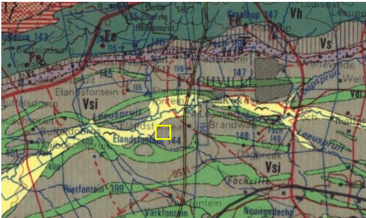
Figure 2: Geological map of the area around Fochville and Kokosi, south of Carltonville. The location of the proposed project is indicated within the yellow rectangle. Abbreviations of the rock types are explained in Table 2. Map enlarged from the Geological Survey 1: 250 000 map 2626 West Rand Parys.
