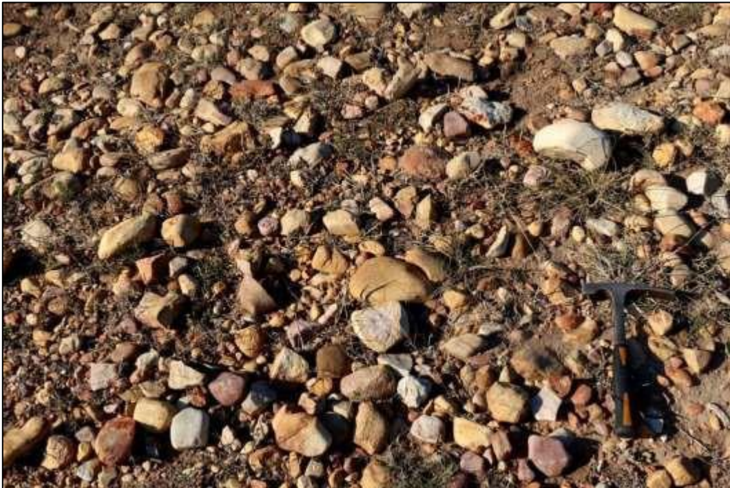
Figure 17: Close-up of pebbly surface gravels near Chatty Substation, predominantly of TMG quartzite and mostly reworked from pre-existing conglomerates of the Alexandria Formation or younger Cenozoic fluvial gravels (Hammer = 30 cm).
