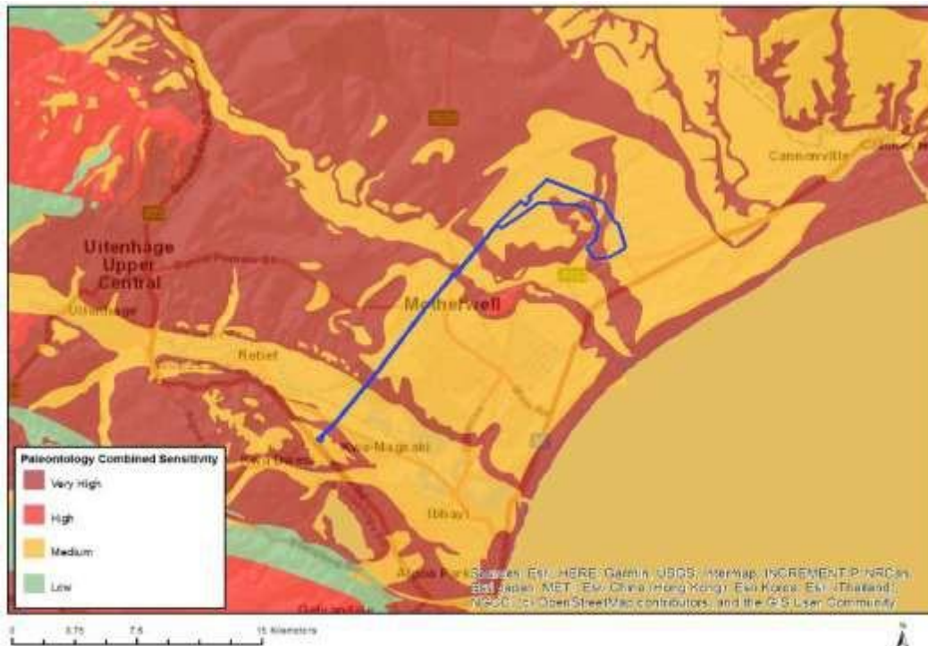
Figure 22: Palaeosensitivity mapping of the Impofu grid extension corridor (blue) based on the DEFF screening map. Dark red areas of Very High sensitivity are underlain by potentially fossiliferous bedrocks of the Sundays River and Kirkwood Formations.
