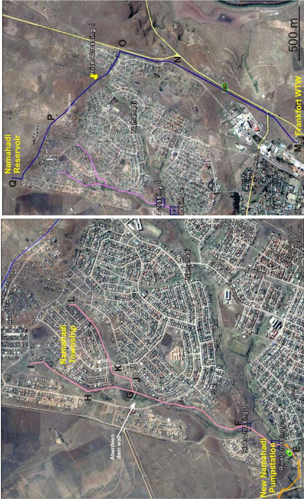
Figure 4. Aerial view of the pipeline footprints between the new Namahadi pump station and the Namahadi Township (left, pink line) and between the Frankfort WTW to Namahadi Reservoir (right, blue line).
