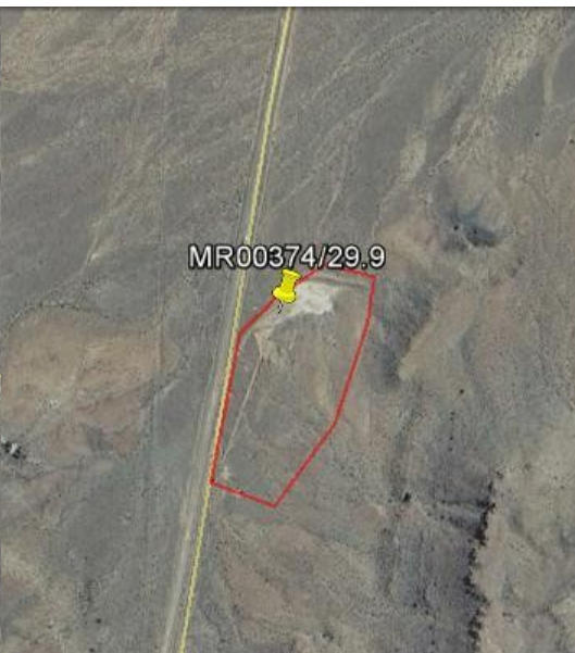
Figure 6: At km 29.9 Aerial view of proposed borrow pit and expropriation area (Google earth image, June 2012)
