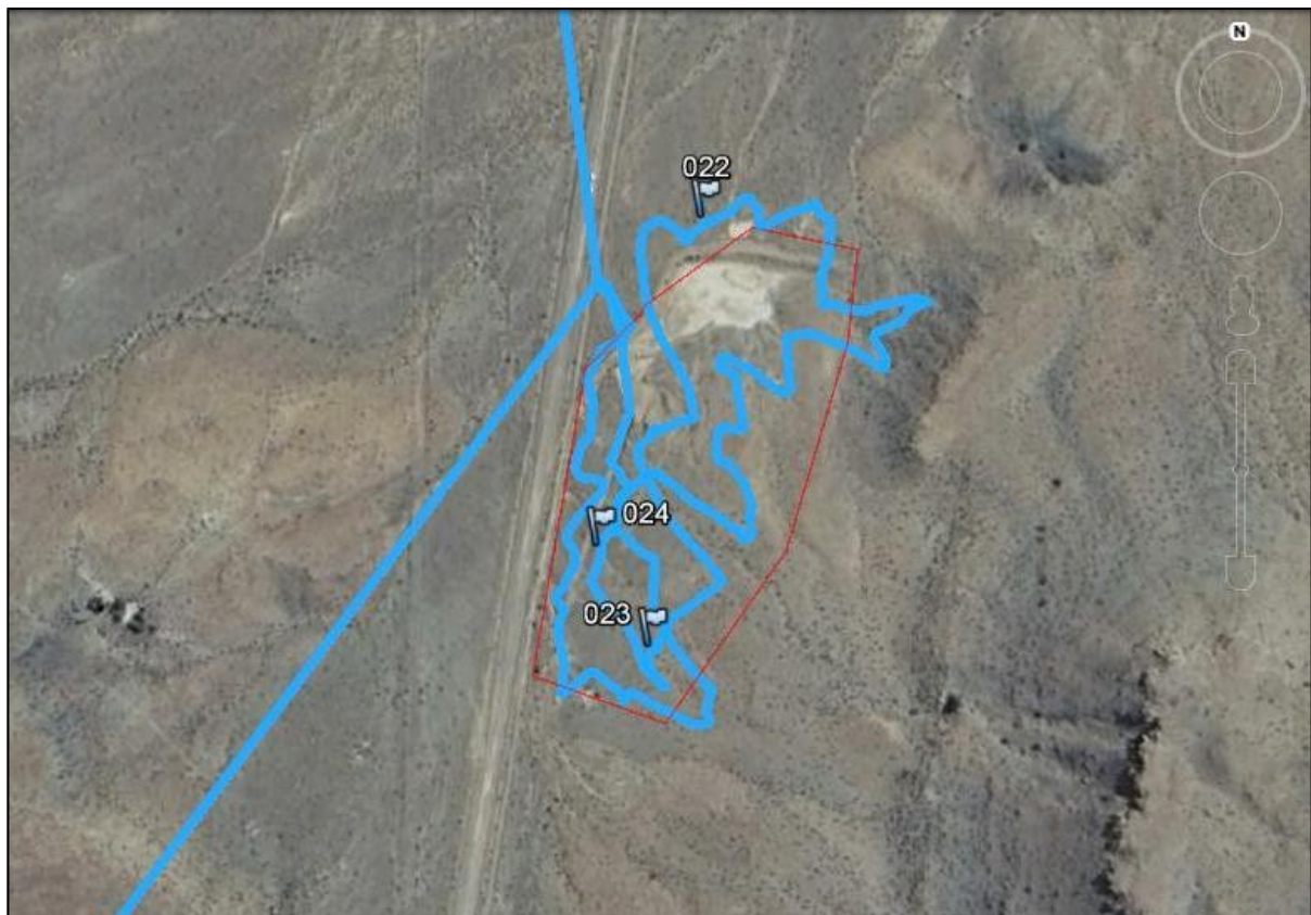
Figure 12: Google earth image showing the proposed extension to borrow pit 112, the tracks and waypoints of the field survey. The western side of the affected area has several channels and small dongas leading water to the existing dam. Please note that the straight blue lines do not indicate survey tracks.
