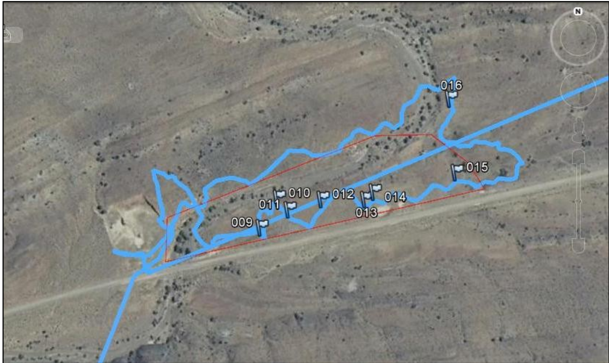
Figure 2: Google earth image showing the proposed borrow Pit 110, waypoints and tracks of the field survey. The small dam to the west of the affected area and the stream bed running through the northern half are evident. The side branch of the stream is close to the south-eastern boundary of the polygon. Please note that the straight blue lines do not indicate survey tracks.
