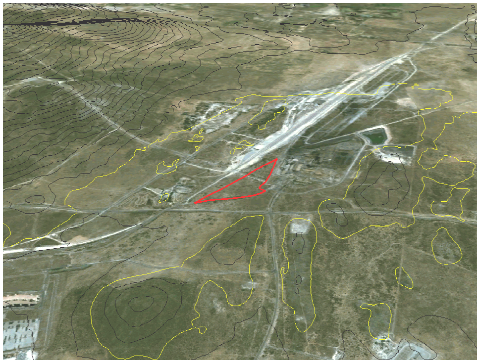
Figure 2. Simulated oblique aerial view of the site, looking north. The study area is shown in red. The 25 m asl. contour is highlighted in yellow. From Google Earth with 5 m contour overlay.
