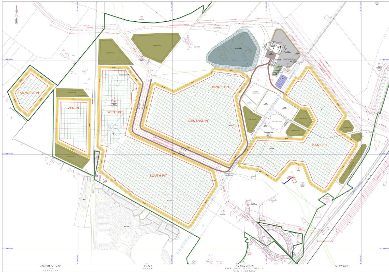
Figure 6 – Mine Layout Plan – Option 2 (provided by uKhozi, Feb 2022) (Overburden and berms-brown, Pit-green, Plant-grey)
