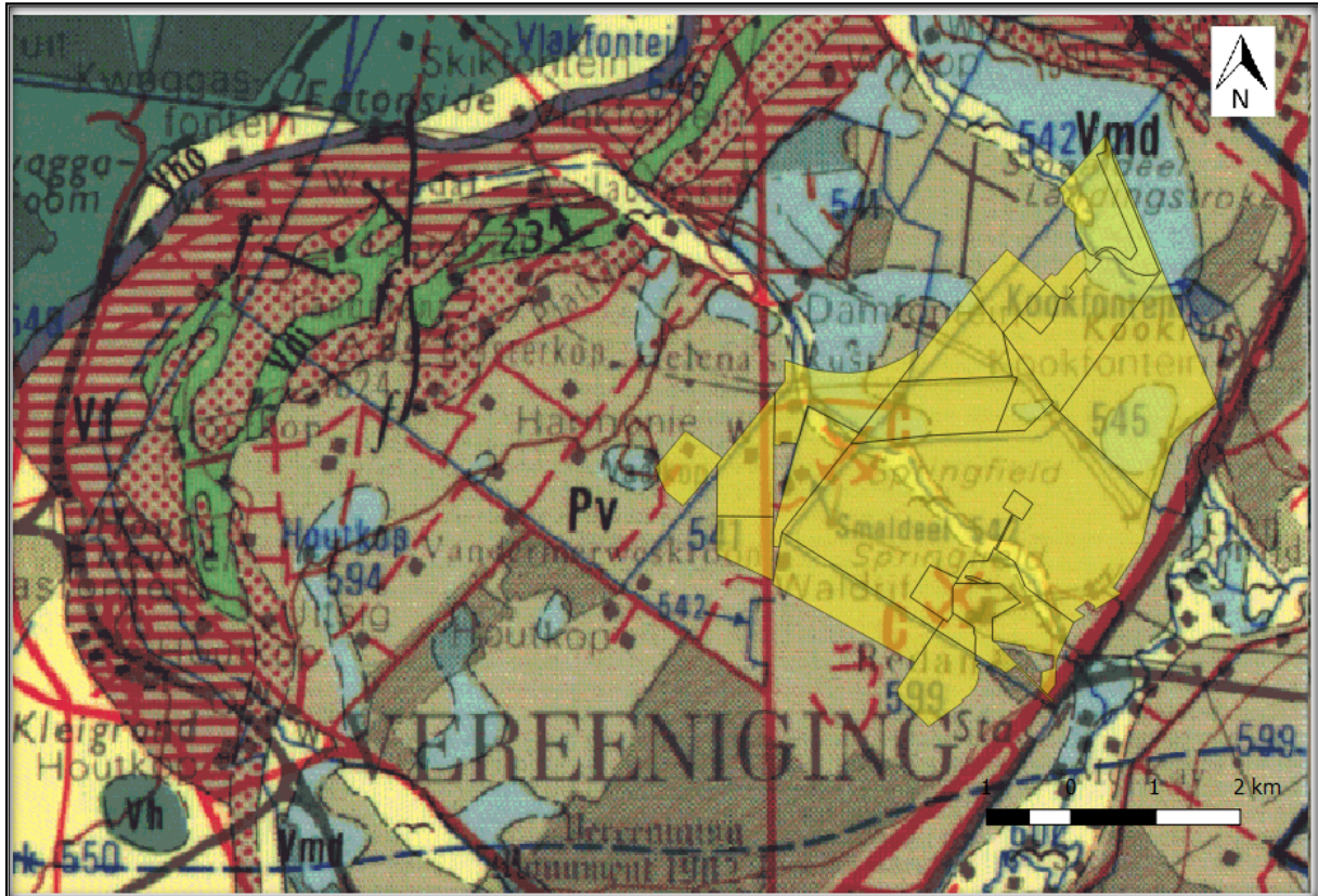
Figure 50 - Extract of the 1:250 000 2626 West Rand Geological Map (Council for Geosciences, Pretoria) indicating the geology of the proposed Springfield Project, between Vereeniging and Meyerton in Gauteng. The Project is underlain by the Vryheid Formation (Ecca Group, Undifferentiated Karoo), Malmani Subgroup (Chuniespoort Group, Transvaal Supergroup) and Quaternary deposits. Map drawn by QGIS 2.18.28.
