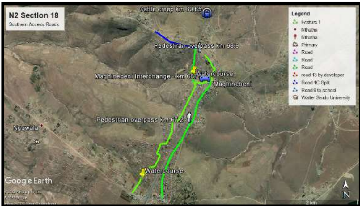
Figure 5. Google Earth Imagery showing the southern section of the project area. The blue and green lines indicate the access roads earmarked for upgrading.
