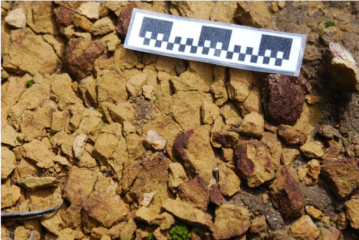
Figure. 7. Crumbly yellow weathered diamictite exposed in a prospecting pit in the extreme east of the study area (Fig. 3 pt.1)
