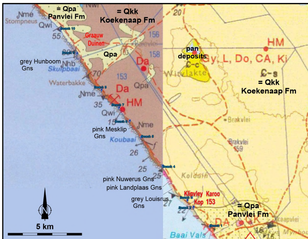
Figure 5-2: Extracts from 1:250 000 sheets 3017 Garies (LHS) and 3118 Calvinia (RHS). Council for Geoscience. Points labelled in red (DA, HM etc.) indicate mineral resources (e.g. Diamonds, Heavy Minerals).
