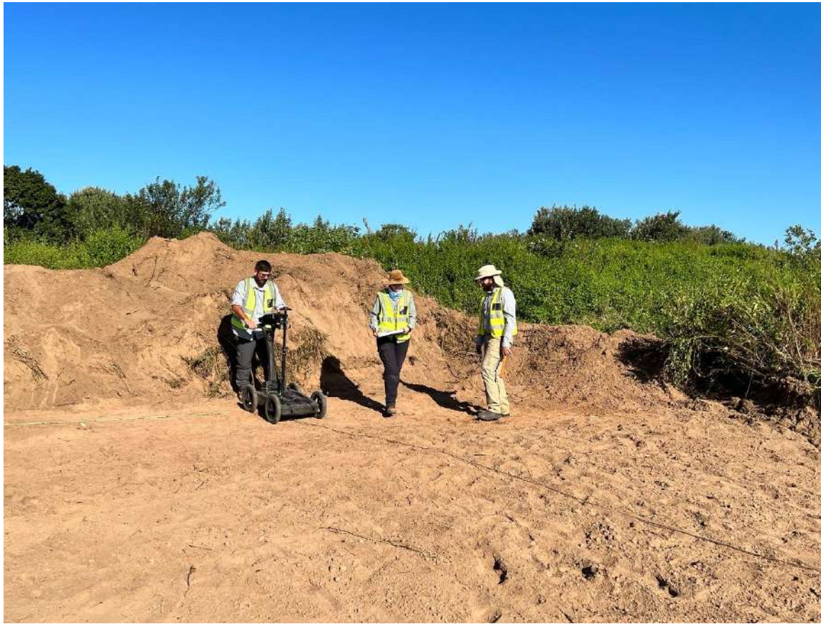
Figure 16 - GPR scanning of the site
