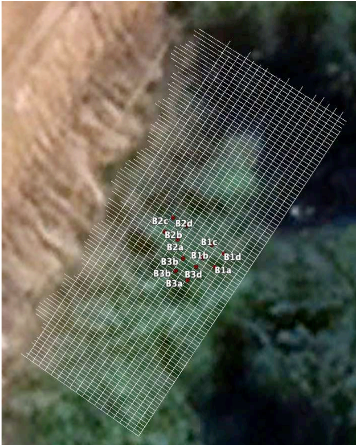
Figure 7 – GPR and excavation grid overlay (Red dots indicate test trench corners)
