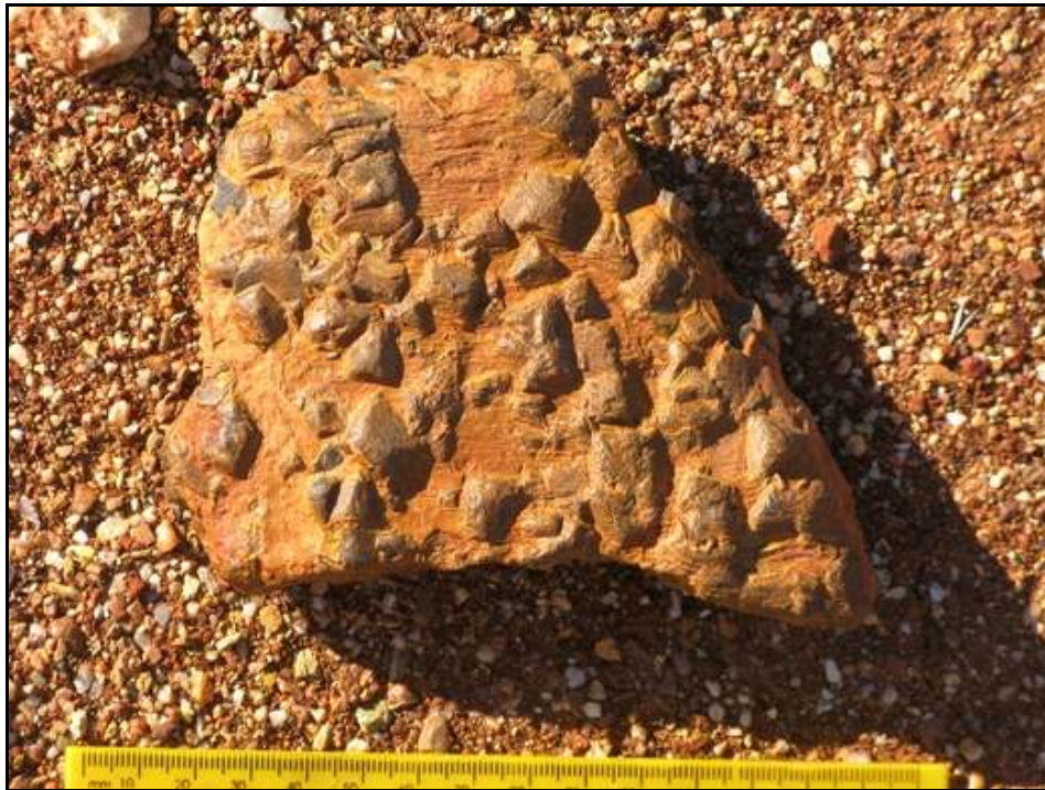
Fig. 8. Ferricrete clast from superficial gravelly deposits showing large cubical pseudomorphs after pyrite crystals (Scale in cm and mm).
