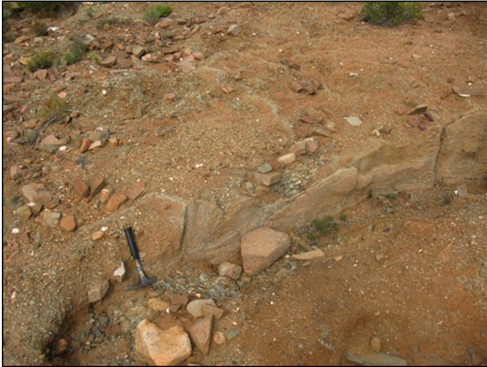
Fig. 7. Penetrative polygonal crack system developed within fine gravelly superficial deposits on the existing pit margin (Hammer = 29 cm).
