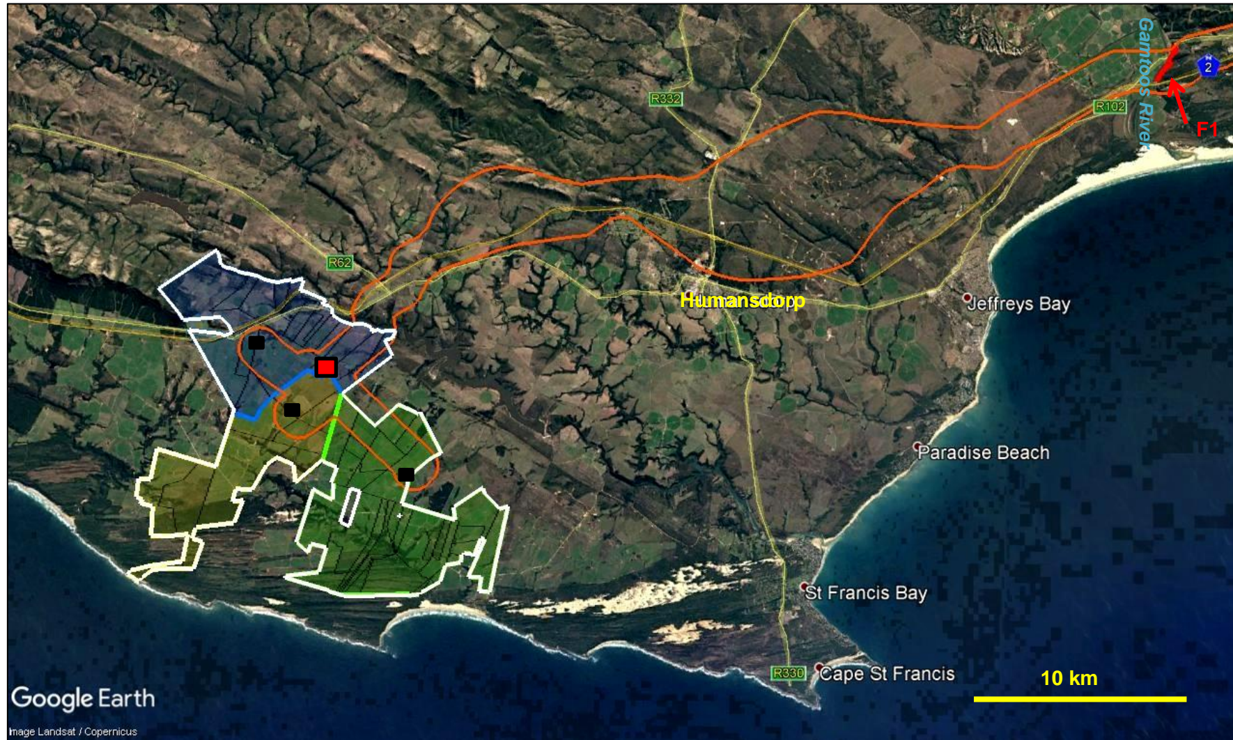
Figure 1. Google Earth© satellite image of the western sector of the Impofu Wind Farm 132 kV grid connection corridor study area (orange polygon) extending from the proposed new Impofu collector switching station (red square) and the Garmtoos River, Eastern Cape. The three switching stations (black squares) connecting to the central collector switching station as well as the combined Impofu North, Impofu East and
