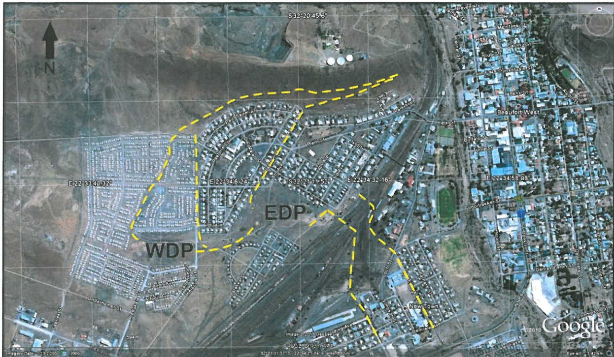
Figure 2. Aerial photograph of site (current), Western Detention Pond (WDP), Eastern Detention Pond (EDP), and associated earth channels (in yellow) of the proposed development in Hillside, Beaufort West, Western Cape.
