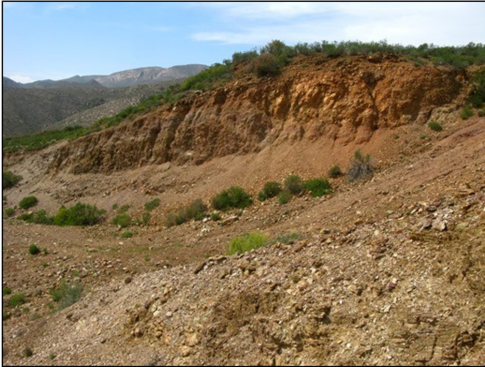
Fig. 4. View towards the southeast of the existing pit DR01347/17.22/L/500/A/W3 showing weathered micaceous siltstones in the foreground and brown-weathering sandstones of the Floriskraal Formation in the cut face behind.
