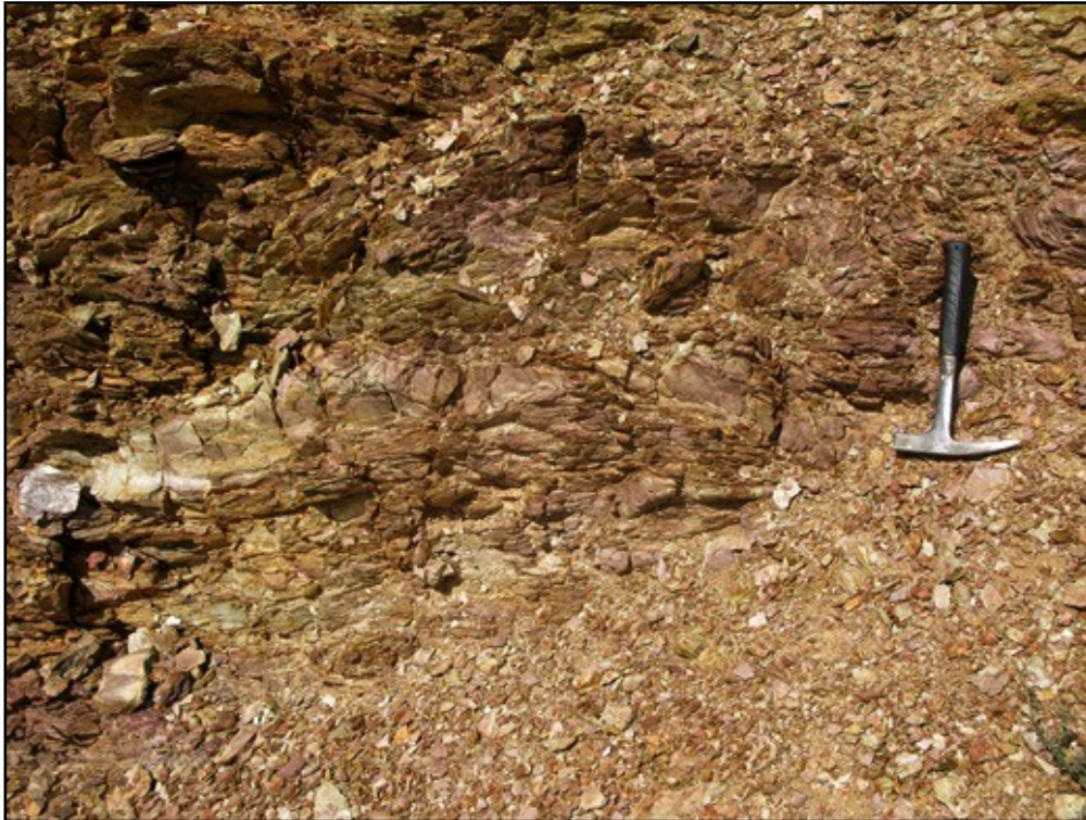
Fig. 6. Highly disrupted, tectonised micaceous wackes and siltstones in pit DR01347/17.22/L/500/A/W3 (Hammer = 30 cm).
