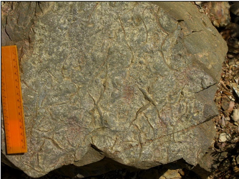
Fig. 13. Sandstone bedding plane from the Floriskraal Formation in pit DR01347/17.22/L/500/A/W3 showing irregular, spindle-like synaeresis cracks, often mistaken for trace fossils (Scale in cm and mm).
