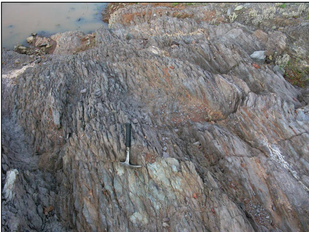
Fig. 5. Greyish siltstones and wackes of the Adolphspoor Formation exposed on the steep SW face of the pit showing pervasive steeply-dipping spaced tectonic cleavage (Hammer = 29 cm).
