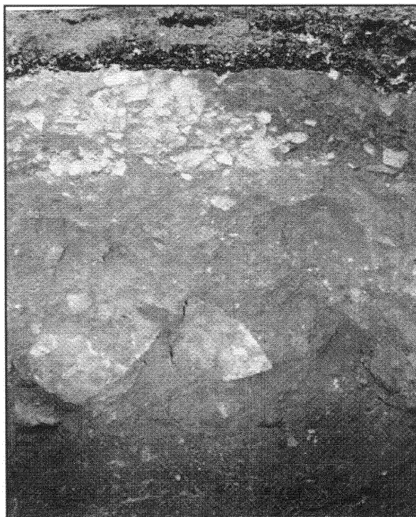
Plate 2: Section of Hole 1 showing the tarmac, gravel sub-base and mixed rubble, rocks and clay.
