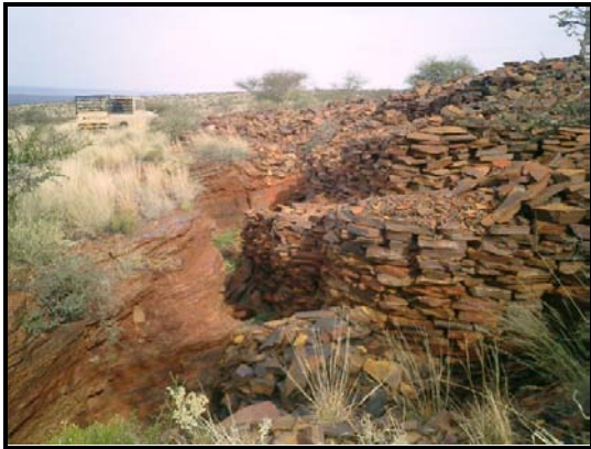
IMAGE 3: Close-up of the proposed mining area indicating the method of stepped rehabilitation (right) while mining is in progress and the basal banded ironstone reaching to the surface of the hill (left)
