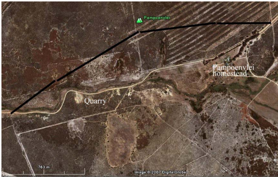
Figure 2. The realignment road section (black line) will be to the north of the existing road to avoid further damage to sensitive vegetation along the river.
