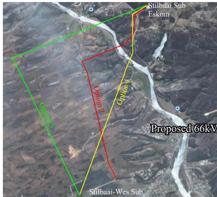
Fig. 2. Three options proposed by the land surveyor. Option 2 is the preferred route.
