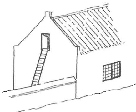
FIG.22 Access was gained to the loft via the end gable AA1 by means of a ladder.
