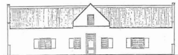
FIG.21.1 The dwelling may have acquired a simple central gable (a) (Fagan & Fagan 1974), or a more elaborate one (b) (Vos).
