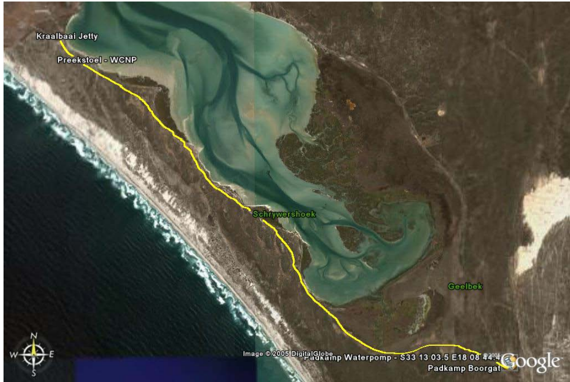
Figure 2. Aerial photograph of the study area. The yellow line indicates the route that the pipeline will take from 'Padkamp' near Geelbek, to the proposed rest camp site at Kraalbaai, a distance of 15.8 km.
