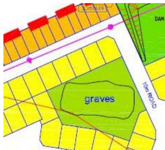
Fig. 7. The development plan shows a buffer zone in green around the graves. The buffer zone in the northeast corner of the cemetery is limited and it is important to ensure the graves are not impacted by road or other development.
