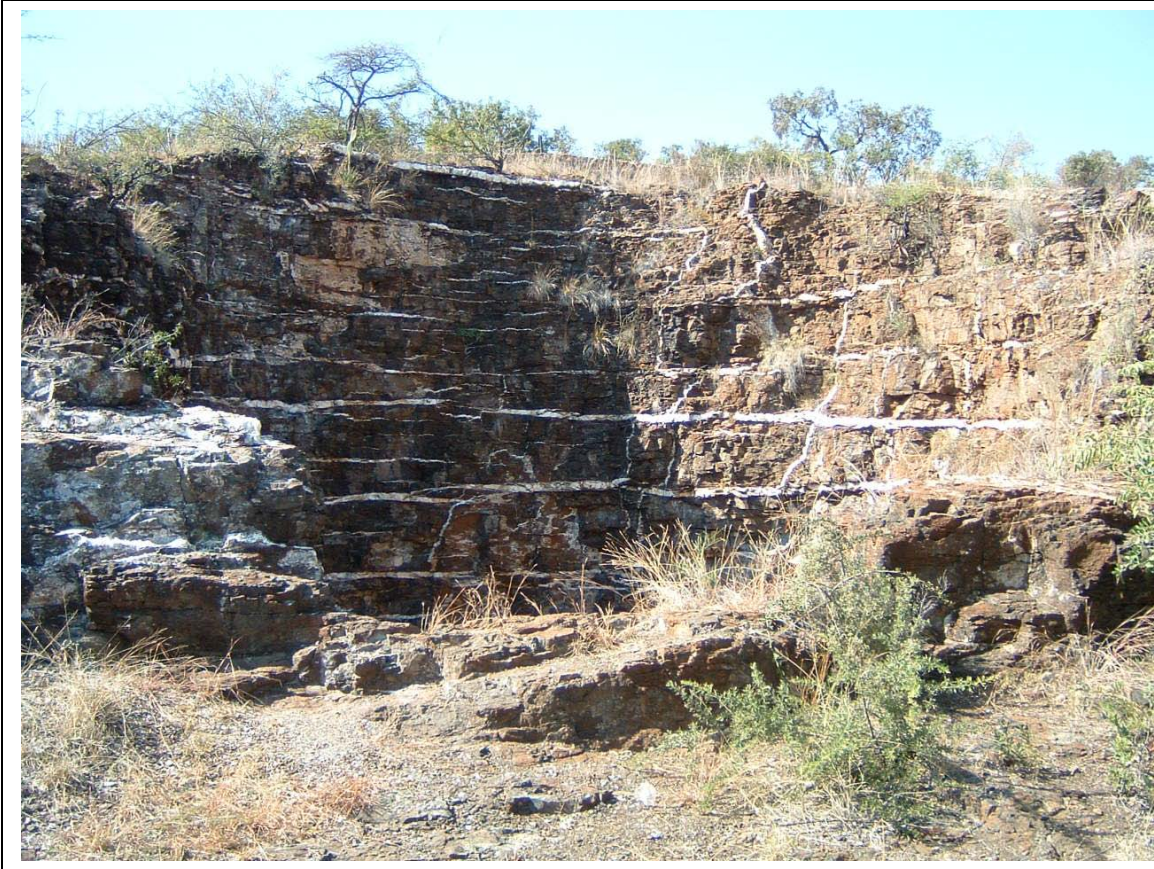
Figure 11- Side wall of the Onverwacht platinum ‘pipe’ showing the hortonolite-dunite walls of the open mine which is traversed by a roughly rectangular network of magnesite veins up to 9” in thickness. These white veins strike a sharp contrast against the surrounding dark rock.
