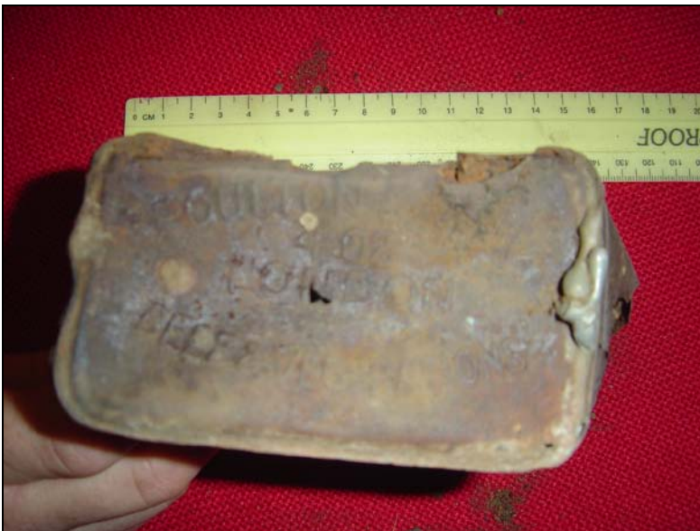
Fig.37 Food tin inscribed: PAULTON & NOEL 402 LONDON BEEF & VEGS. RATIONS. Note the coarse soldering on the rim.
