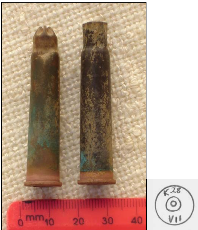
Fig.14 Unfired and fired ,303 blank cartridges with head stamps inscribed K28, Mk VII.
