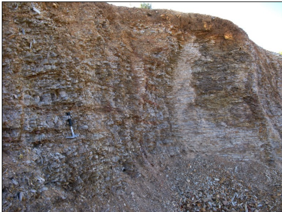
Fig. 7. Cut face of weathered and highly cleaved, pale grey mudrocks of the Whitehill Formation (Hammer = 27 cm). The bedding here dips very steeply north (towards the observer) while the more prominent cleavage is subhorizontal.
