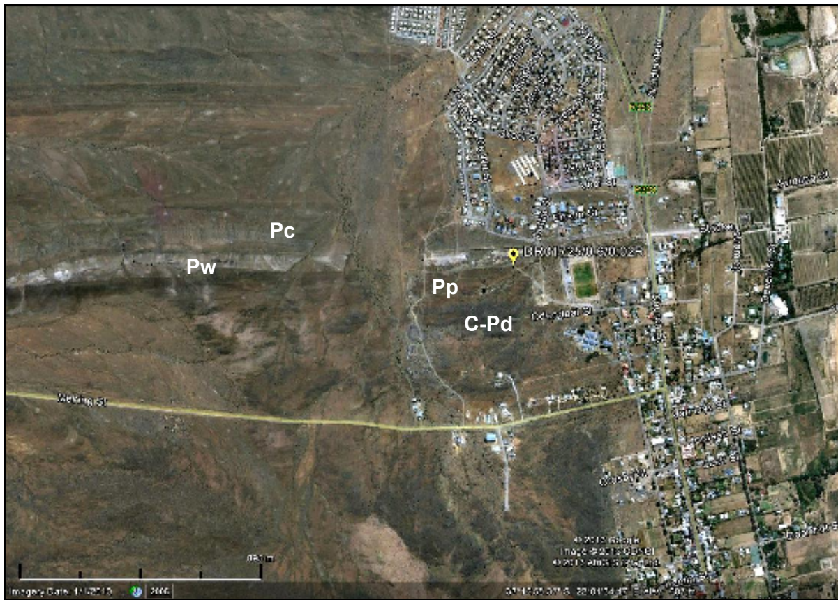
Fig. 2. 2005 Google earth© satellite image of the study area in the Prince Albert Townlands showing the location of the large existing DR01725/0.6/0.02R borrow pit along the DR1725 (yellow symbol). Note the east-west striking outcrop areas of the Dwyka (C-Pd), Prince Albert (Pp), Whitehill (Pw) and Collingham Formations (Pc) as well as the minor stream running N-S on the western side of the pit.
