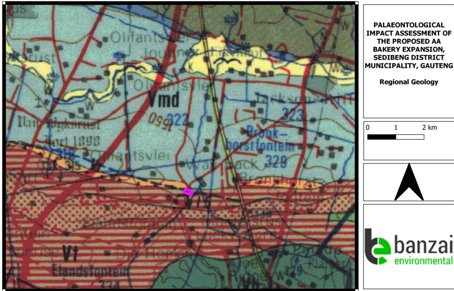
Figure 4: Extract of the 1:250 000 2626 West Rand Geological Map (Council of Geoscience) indicating the proposed development in purple. Surface geology indicates that the development footprint is underlain by the Vaalian aged Timeball Hill Formation (Pretoria Group; Transvaal Supergroup). Map drawn by QGIS 3.10.
