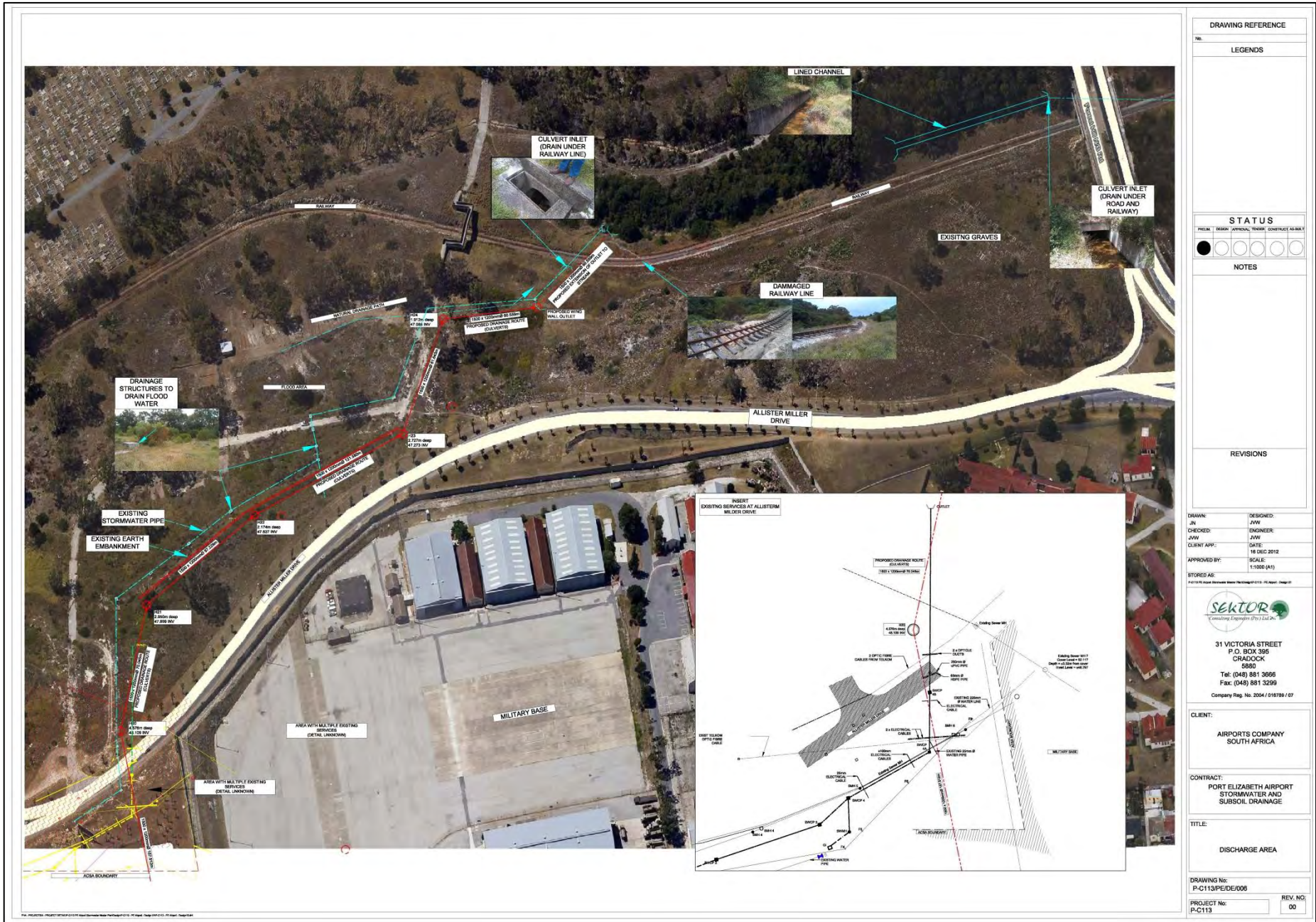
Figure 11. GIS generated map of the layout of the area proposed for the ACSA stormwater outfall system upgrade including the route of the existing pipeline (image courtesy of SRK Consulting).
