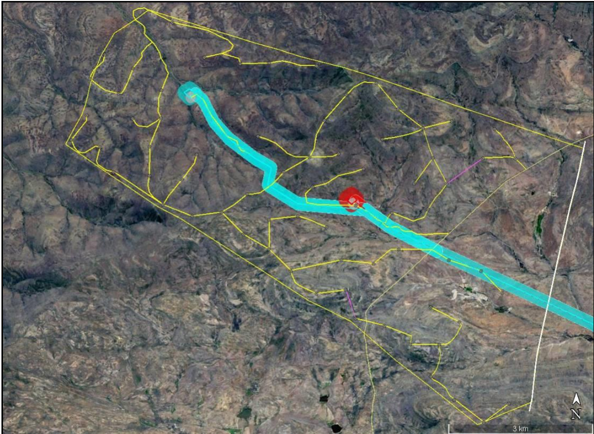
Figure 1: The boundaries of the Maralla West WEF in yellow. They fall within the boundaries of the Northern Cape. The onsite substations are shown in blue and red, and the powerline connection to the substation in blue. Most turbines are placed in the higher ground. The terrain is very mountainous and cabling and roads need to cross valleys and river beds.
