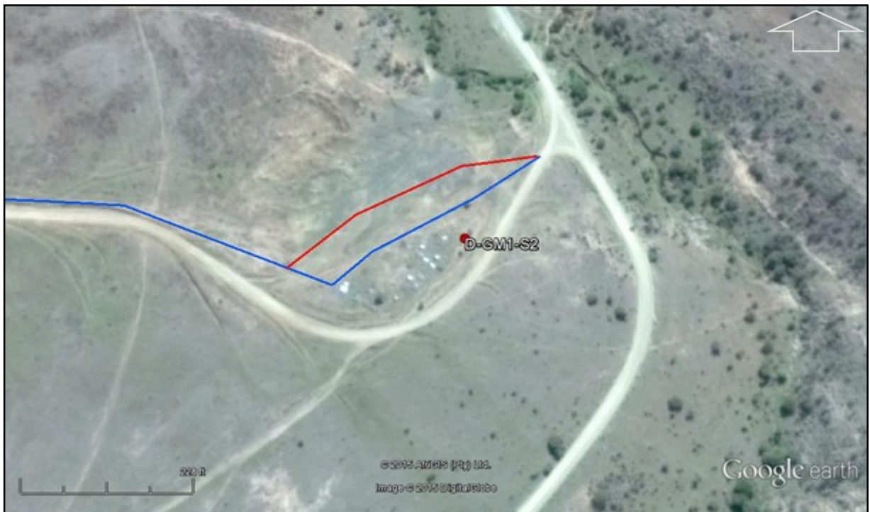
Map 6: Proposed realignment in the vicinity of Site D-GM1-S2 (Blue-Gravity Main 1 alignment; Red – proposed realignment)
