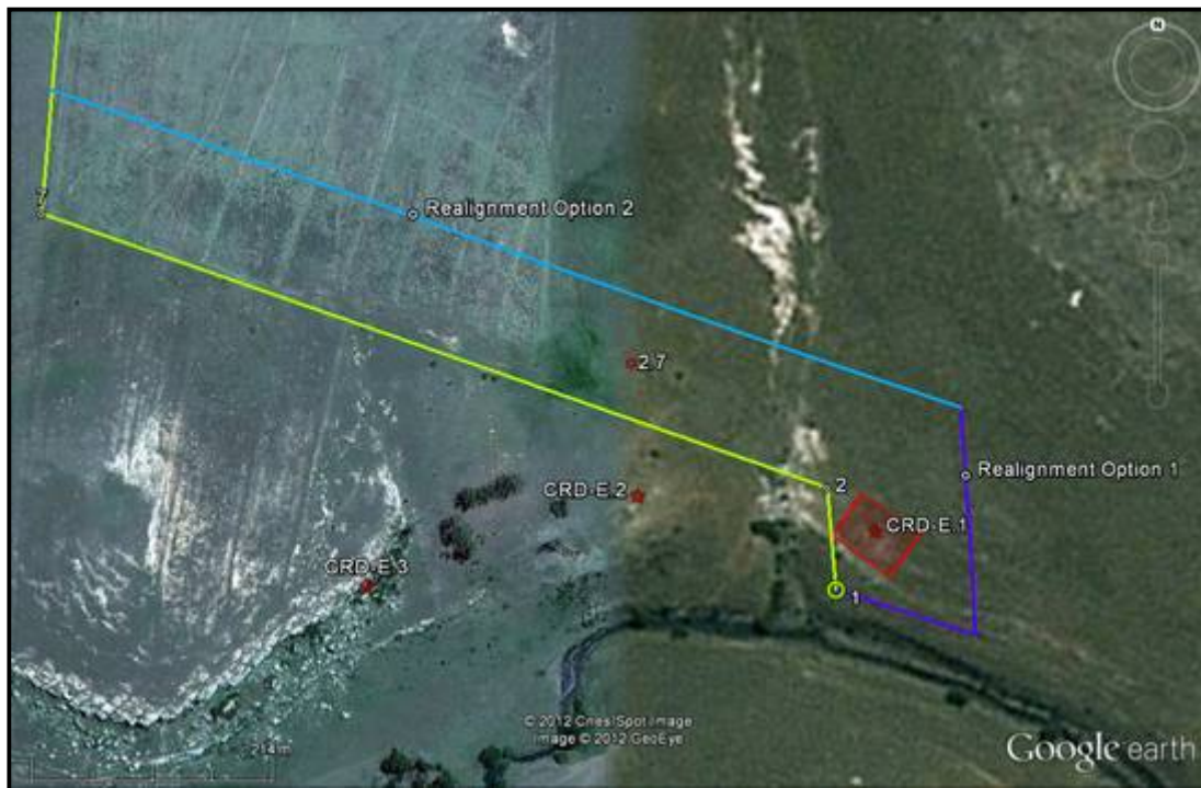
Figure 5: Realignment Option 1 and Option 2 in relation to the current rising main Nodes 1-2-7
