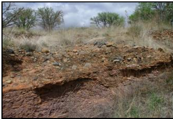
Figure 10: Exposed sections at the STC01 borrow pit clearly indicating the artefact member overlying the shale substrate (no calcrete at this portion of the section)
