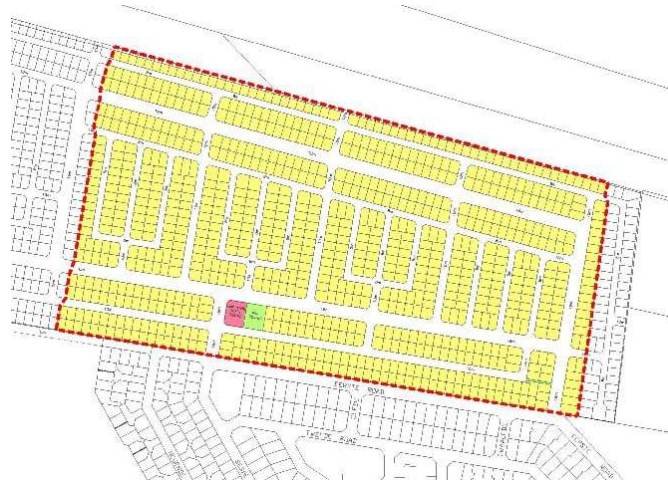
Fig. 3. The draft layout of the proposed low cost housing development with 840 residential erven, mostly 10 m by 15 m in size. The public and community spaces are shown in red and green and together constitute approximately 1% of the area of the development which seems inadequate to promote community well being.
