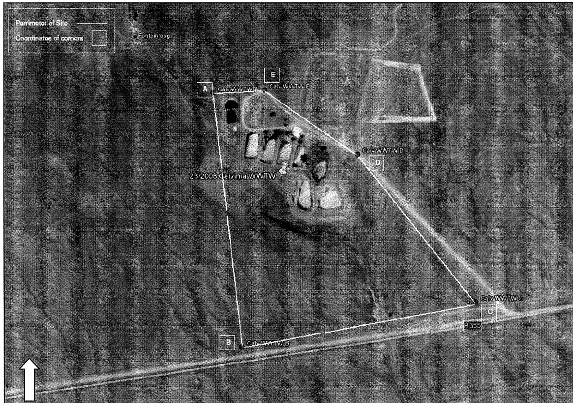
Figure 2: The borders of the proposed extension to the Calvinia WWTW after Van Zyl Environmental Consultants cc. The location of the fountain is marked to the north-west of the site, while the location of the municipal dump is visible to the north-east. The drainage area below the oxidation dams is clearly visible.
