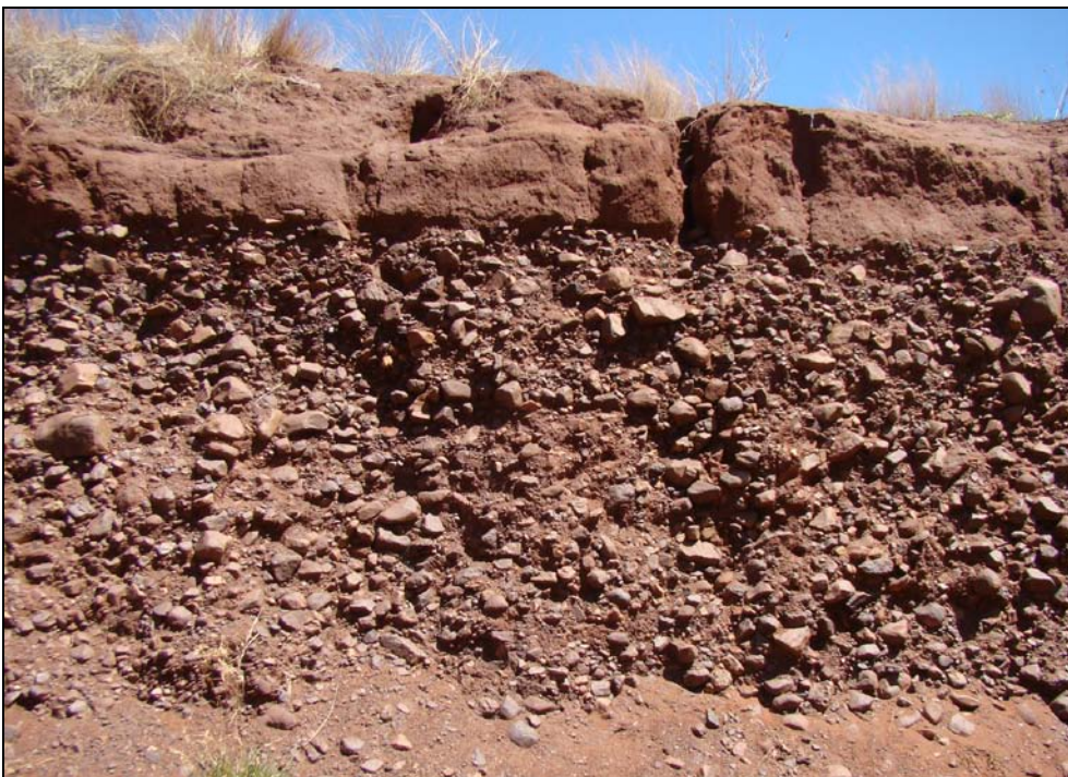
Fig.17 Profile of test pit in alluvial deposit in the Gamogara flood floor.
