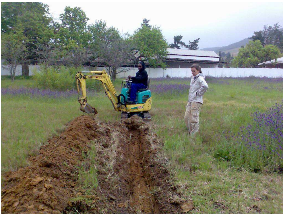
Plate 1 Checking the status of sub-surface soils using a micro-excavator.
