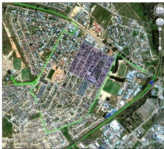
Figure 6: Proposed deviation to repeater (green line) in Wesbank, Malmesbury. The area shaded purple has been identified in the Swartland Heritage Survey as a Special Area and is associated with the development of Wesbank as a suburb of Malmesbury during the Apartheid era. The proposed cable in the road reserve will not impact on any buildings (SHSG 2009).
