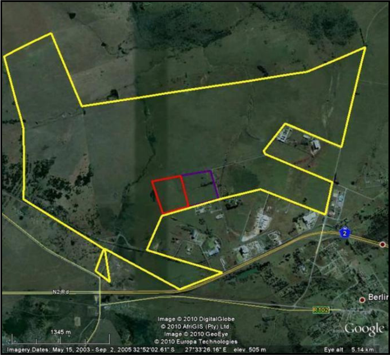
FIG. 2: AERIAL OVERVIEW OF THE LANGA SOLAR ENERGY FACILITY. THE RED AND PURPLE AREAS ARE EARMARKED FOR THE 10MW PILOT.
