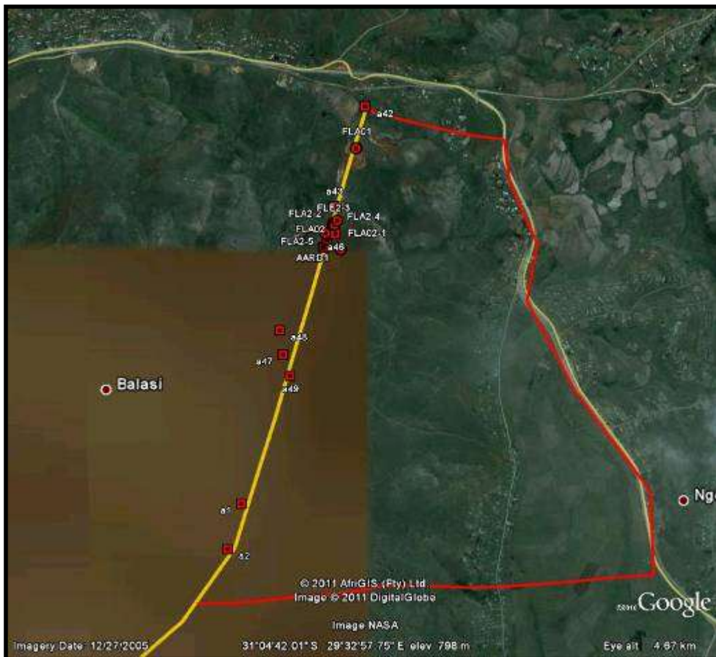
FIG. 28: EXISTING AND PROPOSED TRANSMISSION LINE ROUTE 7
