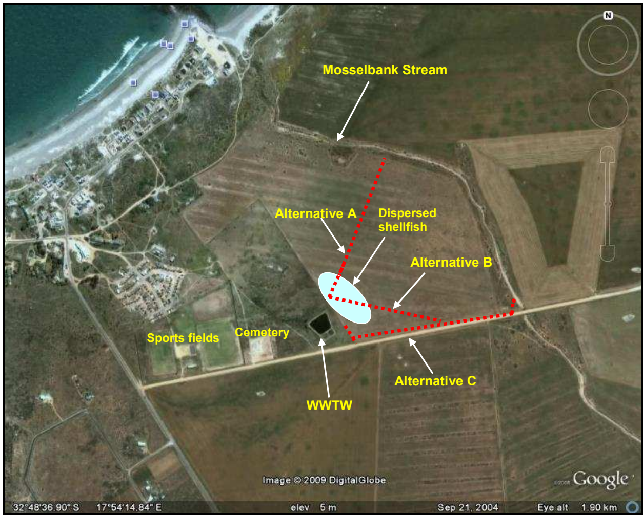
Figure 2. Aerial view of the study site and the proposed (A) and proposed alternative (B & C) pipelines
