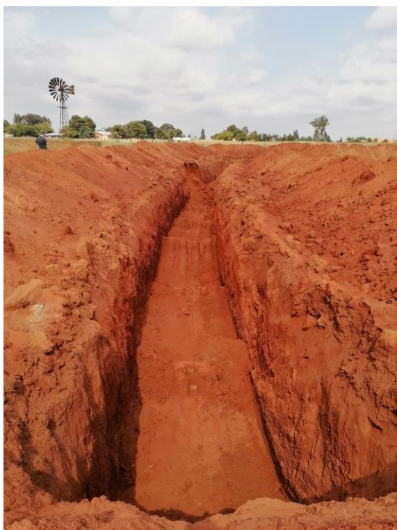
Figure 21: Deep excavation indicating depth of sandy topsoil and absence of any geological structure
